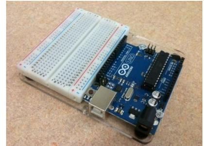
Arduino Uno R3 and half-sized breadboard.
